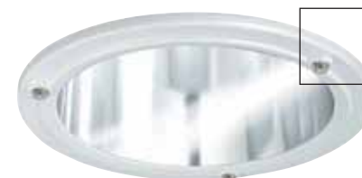
DOT A31-CL Clear Lens IP54 Polycarbonate flush mounted c/w Tri-groove tamper proof fasteners – 275mm dia. /01 White trim /55 Silver trim
