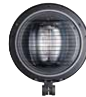
Matt Black aluminium louvre mounted inside the luminaire for limiting glare and increasing visual comfort. To suit curved glass and Acrylic visors only. - Louvre Option
