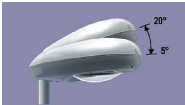
Post-top suitable for 60-62mm diameter column with adjustable upcast 5° & 20°
