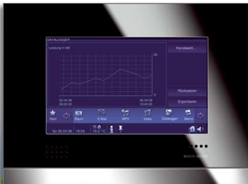
Graphical display of the consumption values in the Busch ComfortPanel
