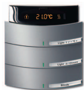
3-fold control element with rear-illuminated labelling field, integrated room thermostat without IR reception
