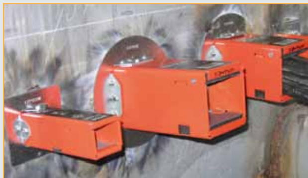
Metallic partitions in the WFR test wall
