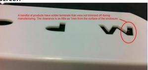
There exists a manufacturing fault where a small number of products have untrimmed input power terminals, located at the underside of the control box. Our internal review shows that there are approximately 1 in 25 products with the defect. The untrimmed terminals could potentially extend to, or close to, the surface of the underside of the control box, where a small ventilation cavity exists.
