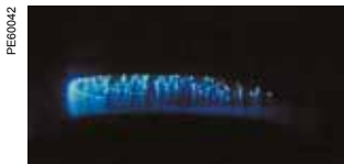
Fig. 3: diffuse vacuum arc AMF technology
