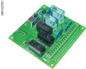
Control card for the switch-disconnector gear motor
