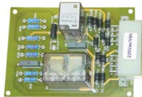
Control card for circuit breaker spring charging motor
