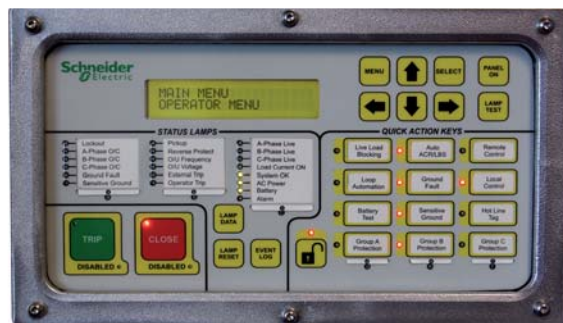
flexVUE Operator Interface
