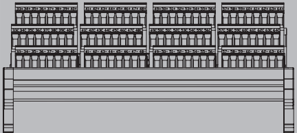
Field terminals view for ADV161 (Channels 33 to 64)
