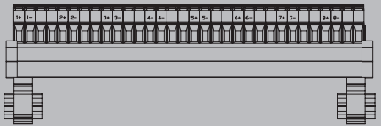
Field terminals view for SAI533
