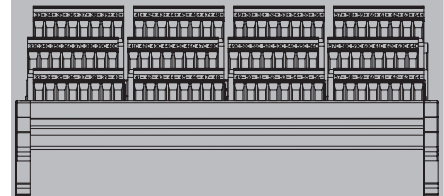
Field terminals view for ADV161 (Channels 33 to 64)
