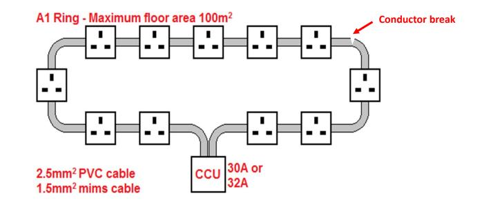
**Note.** This only applies to a series arc fault in a ring circuit not a parallel arc fault.
