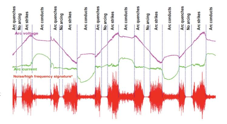
Noise / high frequency signature exceeding 50 Hz which can be kHz or MHz and which correspond to an electric arc fault
