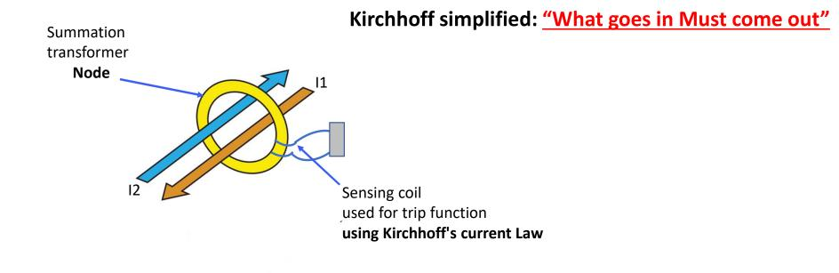
Note: RCD's do not measure what current is flowing into the circuit protection cables to earth!
