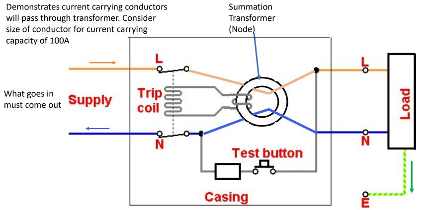
Leakage current mA somewhere in electronic circuits. Insulation failures leading to earth fault.
