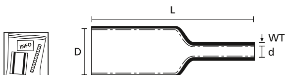
Heat Shrinkable Tubing 4:1 with adhesive
