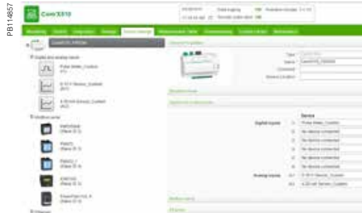
Device settings page (partial), as displayed after auto-discovery, enabling user to assign circuit identifications and select data for logging and publication.
