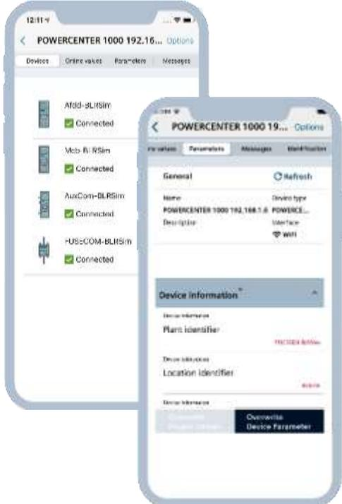
This panel shows a smartphone app interface displaying a list of connected devices: Afdd-BLRSim, Mcb-BLRSim, AuxCon-BLRSim, and FUSE-COM-BLRSim. A detailed view of a device shows its name, IP address, and device type.
