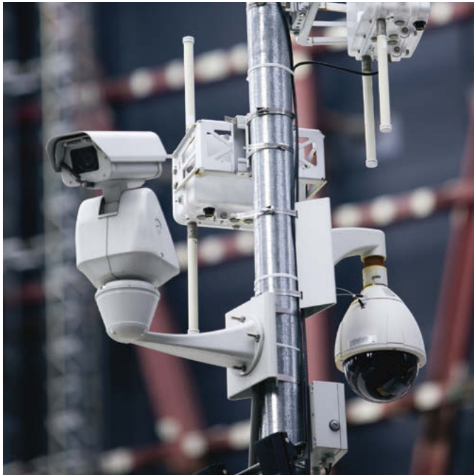
Due to high data transmission rates, surveillance cameras for quality control or plant monitoring are the perfect application for industrial PoE switches with 9.6 kB jumbo frame support. Complex cabling is not required here, as both data and current are transmitted via a standard cable.
