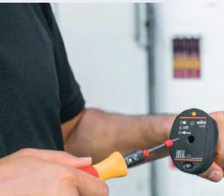
Mobile checking of torque tools
