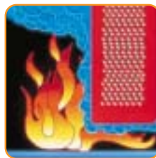
2 nd anti-fire effect: Barrier of water vapour
