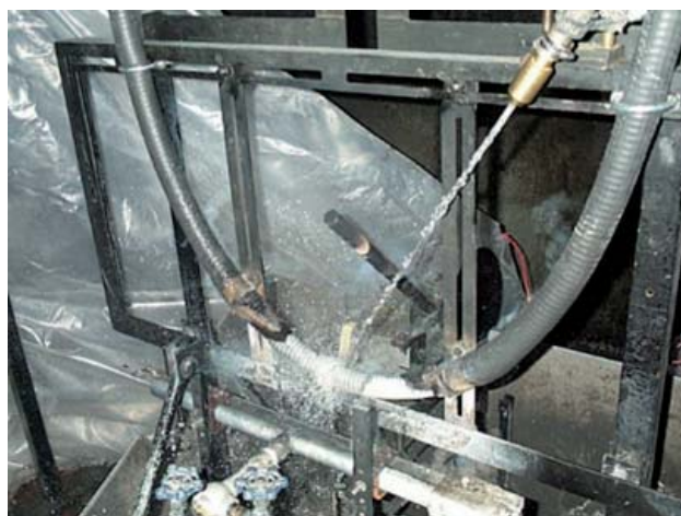
Prysmian FP600 undergoing testing to BS7346-6
