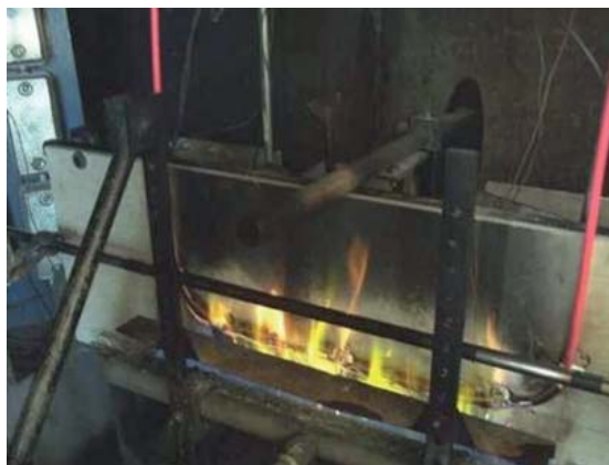
Prysmian FP200Gold undergoing testing to 60 minute requirement of BS EN 50200
