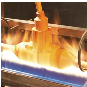
BS6387 Category W - Resistance to fire and water; 650°C for 15 minutes, then for 15 minutes with fire and water
