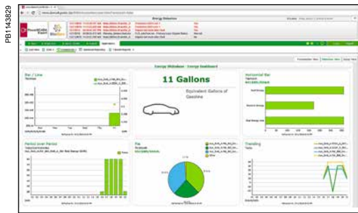
Dashboard di EcoStruxure™ Power SCADA Operation
