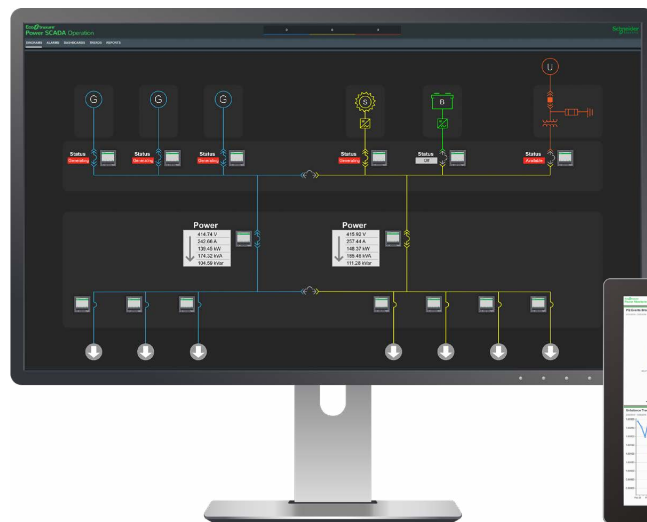
EcoStruxure Power SCADA Operation
