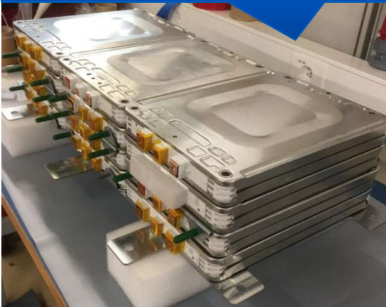
1 Battery String – 12 modules
