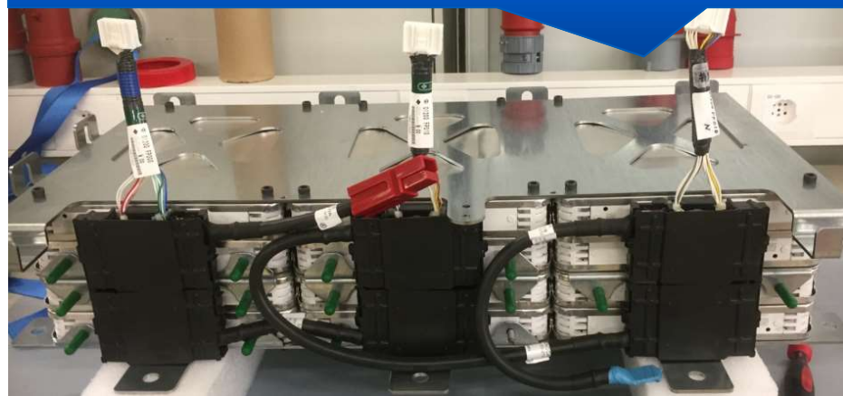
12 modules connected via BBM
