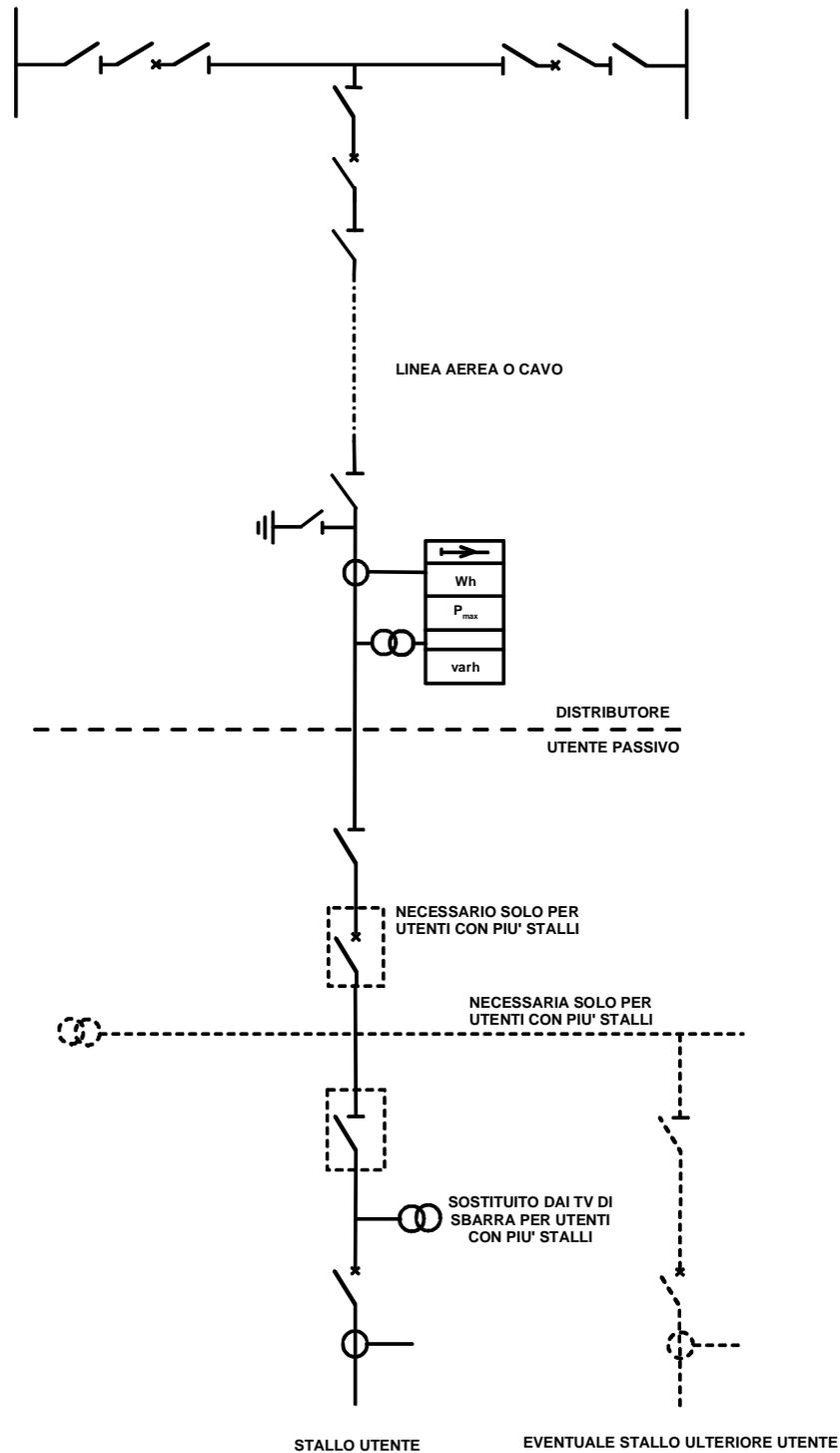
NOTA - 1) IN ASSENZA DI DISPOSITIVO GENERALE (DG), SONO AMMESSI FINO A TRE STALLI ED E' AMMESSA UNA SOLA TERNA DI TV SULLA SBARRA UTENTE.
