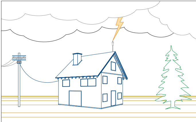
Lightning strike on an external air terminal or on the building
