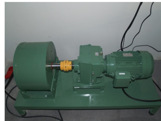
3kW wind micro-turbine emulator
