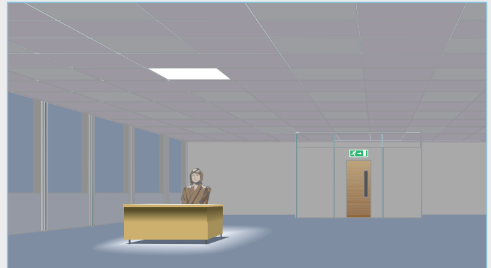
Luminaires which don't communicate cause small pools of light surrounded by intimidating darkness
