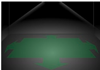
Room illumination with symmetric optics
