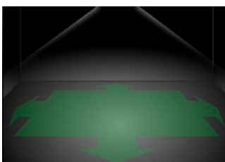
Escape route illumination with symmetric optics
