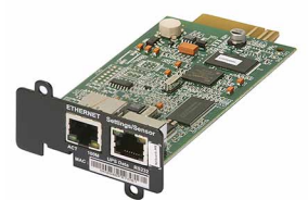
Optional Web/SNMP card with EMP probe for temperature measurement of an external battery cabinet or rack.
