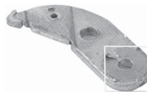
Critical silver-plated surfaces may have plating removed by harsh cleaning methods.
