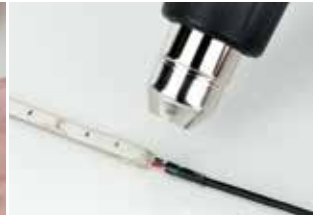
IP Rated LED strip connections heat sealed
