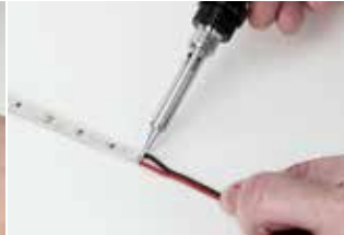
Non IP Rated LED strip cut and soldered to pre ordered length
