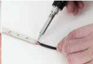
IP Rated LED strip cut, soldered and heat sealed to pre ordered length
