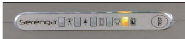
Amber LED indicates a fault Self-test indicator colours may vary
