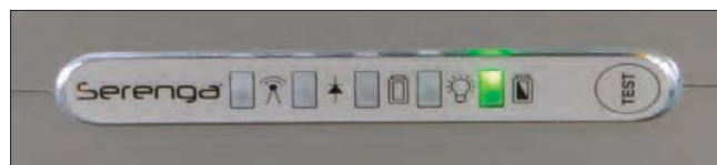
Green LED indicates normal operation
