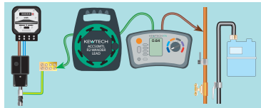
Main Earth Testing
