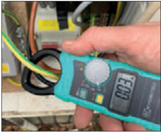
Measures higher level problematical earth leakage currents and also picks up Open PEN situations
