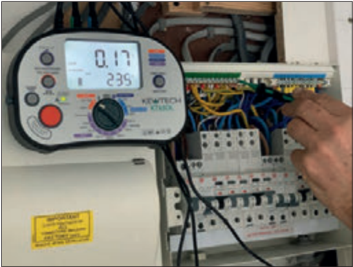
'Hands free' test button for continuous testing and a cleverly designed magnetic base; shown in action.
