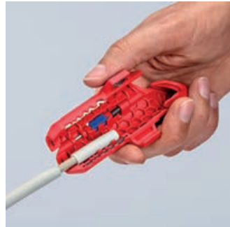
Stripping of a NYM cable
