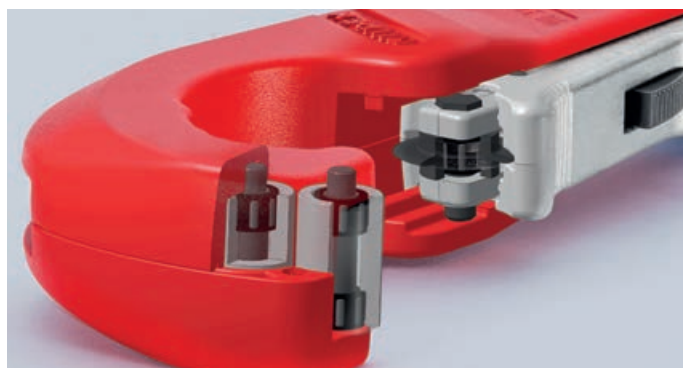
High-quality needle bearings enable the cutting wheel and the four guide rollers to operate virtually without any friction during the cutting – cuts stainless steel pipes with particular ease
