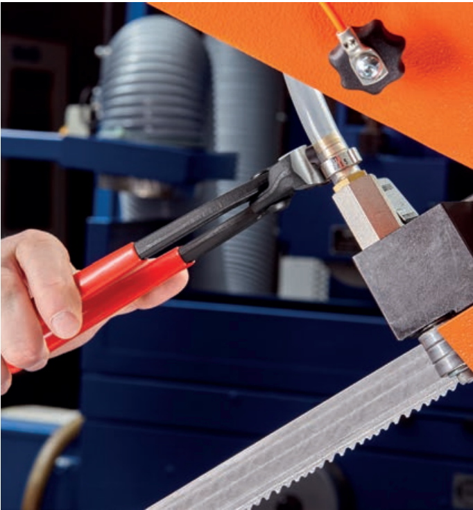
Sealing the fluid hose on the connecting piece using the side press nib
