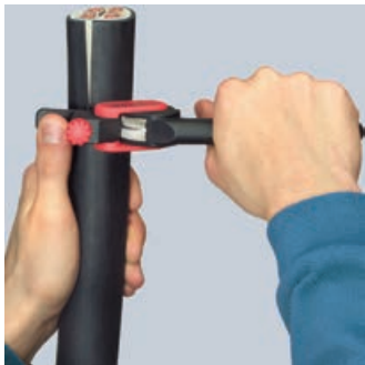
Turning the tool for circumferential cut
