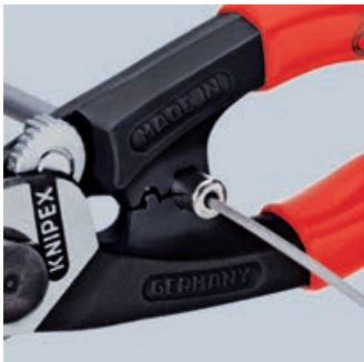
Crimping of the end caps on the Bowden cable sheath
