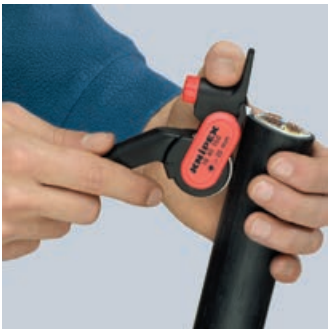
Setting the tool for longitudinal cut
