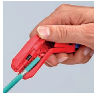
Stripping of a data cable
