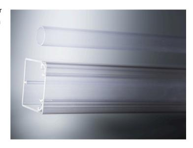
Marshall-Tufflex Maxi data trunking includes a range of slow angle fittings. For this project, 100x50mm clear profiles with flat 90° internal and external bends were used to provide scope for rapid inspection, ensuring that nothing can be concealed within them. 20mm and 25mm clear conduit with terminal boxes and accessories completed the project, with products being manufactured to order in just three weeks over a holiday period.
