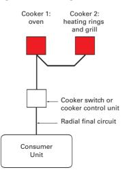
an oven/grill and a separate hob unit), as permitted by Regulation 476-03-04, provided it has sufficient current rating.
