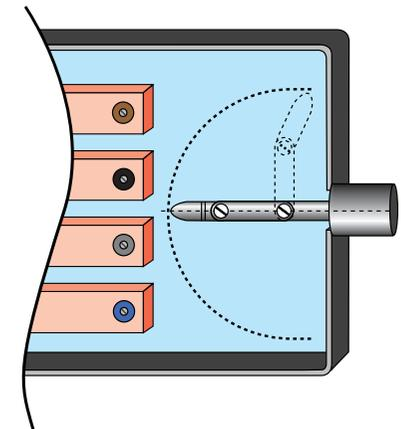
Use of the jointed test finger to establish that an enclosure protects persons against access to hazardous parts.
