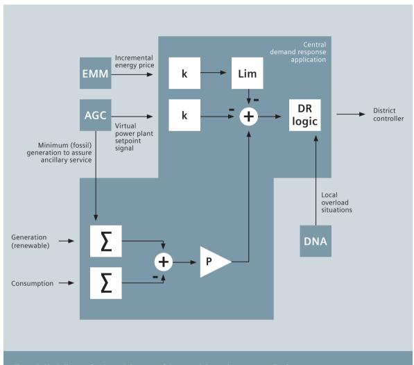
Figure 5: Block diagram for the real-time part of the central demand response application
