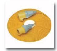
The cable can often be seen supplying caravans or used at live musical events, it can even be purchased from DIY shops in the form of a readymade extension reel with BS 1363 13 A accessories for use at 230 V 1Ø. As can be seen from Table 7B of BS 7540, the cable was not designed for and is not suitable for these purposes.
