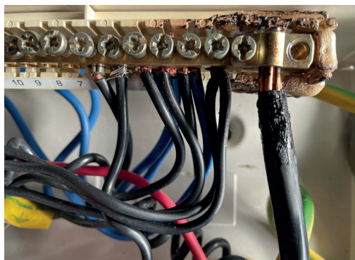
Effects of a loose neutral (image provided by Scolmore).
