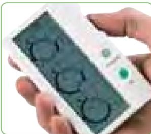
The MB programmer communicates with the heaters and controls a comfort or setback thermostat as per the times set in the programmer.
