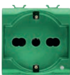
GW 10 224 2P+E-16 A-250 V ac Dual amperage
