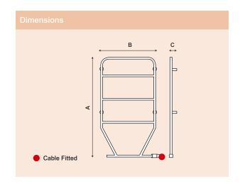
Technical Specification Tubular steel frame | Liquid filled | Cartridge heating element | Thermal cut-out | Chrome or white finish | Fitted mains cable | Supplied with brackets and fixings | All models can be right or left hand mounted.
