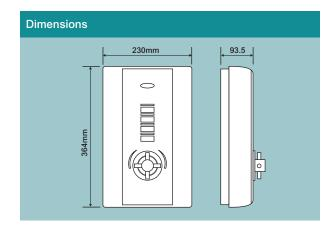
Technical Specification Left or right - Top, bottom or rear entries | Fittings included | Operating water pressure 0.7-7bar (10-100psi) | Water pressure operated power switch | Water connection - 15mm plain shank tails push fit or standard compression fittings. I. Removable lower section. for ease of installation.
