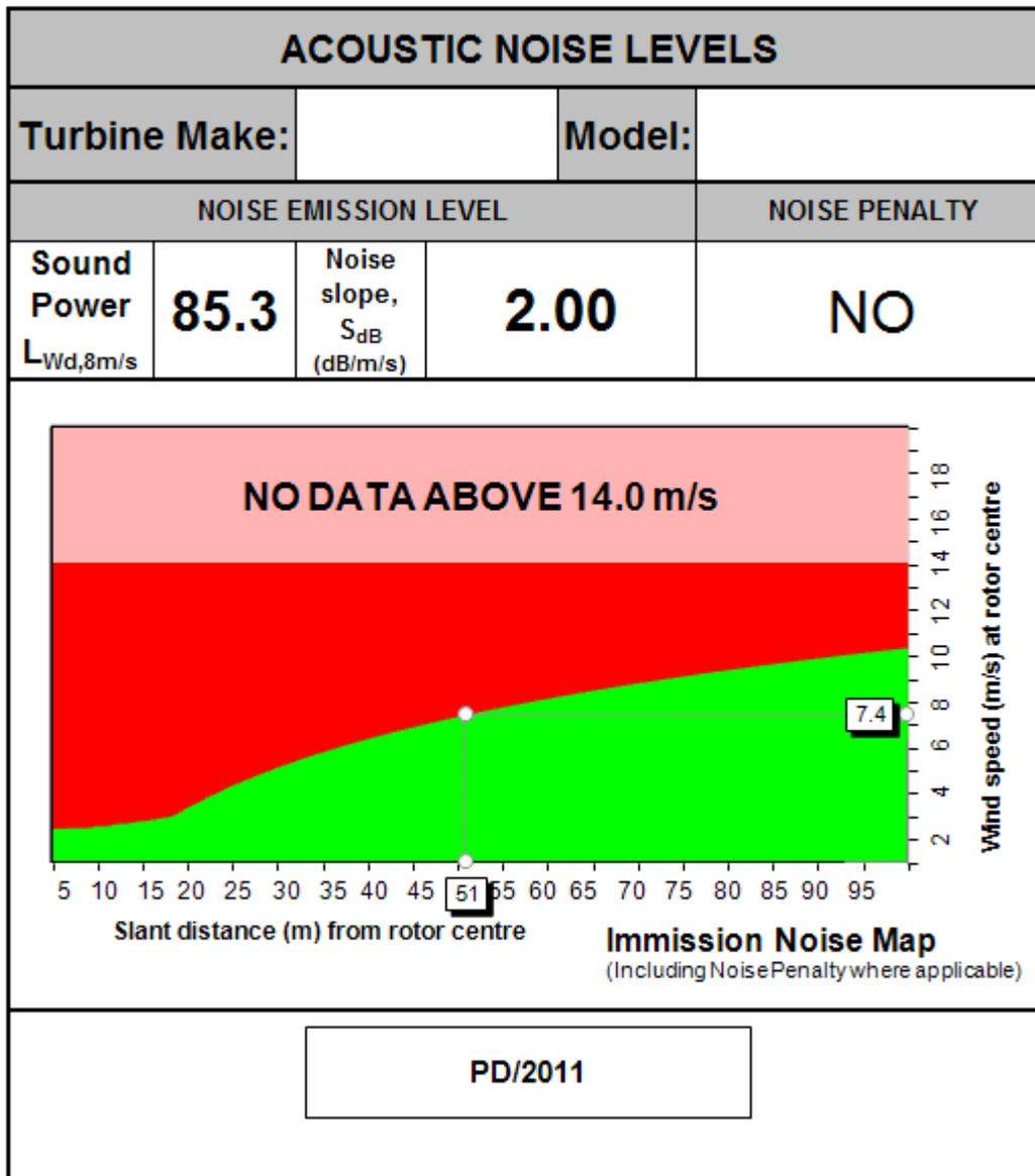
The noise map can be read by drawing a horizontal line from the recorded wind speed at hub (right hand side of the map) to where the red and green lines meet. Drawing a vertical line from this point to the bottom of the map will give the maximum slant distance in metres from rotor centre (hub) at which a wind turbine could be installed to stay within the noise range. For clarity, installers must draw a single line that is no greater than the thickness of a standard biro.
