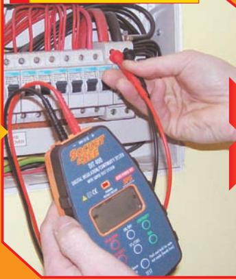
Next, put the probes on the output side, where there should be no indication. (Fig. 4).
