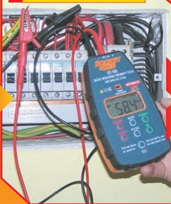
The Socket & See DIT 400 will automatically select the 500V insulation range when you first switch on so just connect your test clips to the conductors to be tested.
