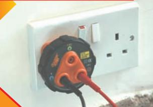
8 Checking for "bridges" at socket outlets
