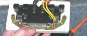
7a Using SS 130 Socket Test Adaptor
